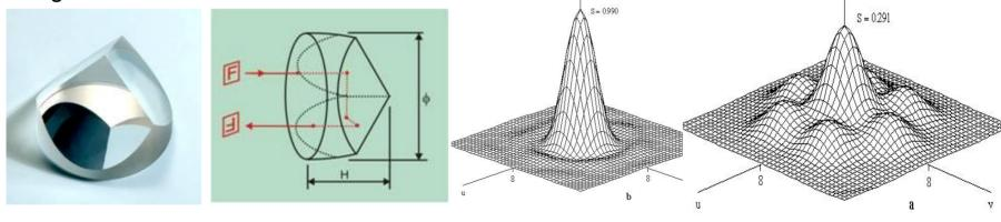
Normalized spatial intensity distributions (u and v are dimensionless coordinates) in patterns of diffraction of unpolarized light by a usual ideal total internal reflection retroreflector (a) and the optimized reflector of the same type having extremely low (diffractional) divergence of a reflected wave (b).
